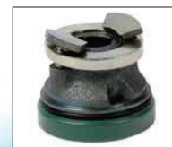
Kingsbury type thrust bearing unit consisting of tilting pads made of highly-resistant stainless steel and machined using the spherical lapping process. From 0,5 HP to 1,5 HP: 2000N (3000N in the 1,5 HP 60Hz version)
