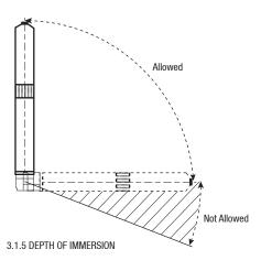
The maximum depth of immersion for all motors is 650 Ft. (200 m)
